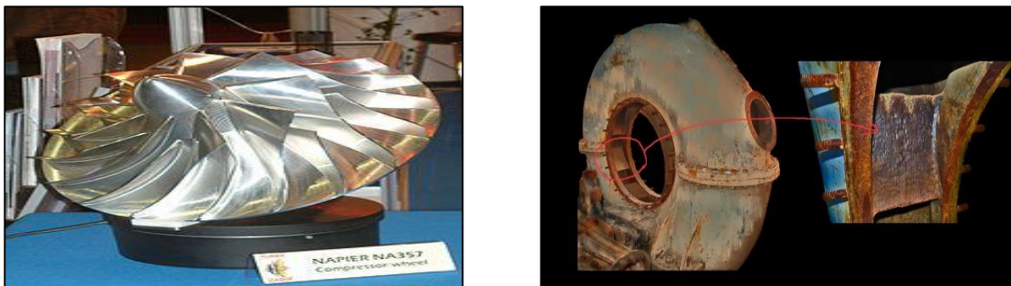
Fig. 9. Compressor Blades and Cavitation in Francis Turbine
